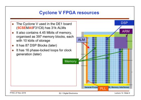
Now let us turn to the Cyclone V FPGA. The FPGA has many different type of resources in additional to Adaptive Logic Modules (ALMs). These are: memory blocks, Digital Signal Processing (DSP) units, phase-locked loops and input/output pads. In addition, there is a dual-core ARM processor and its associated bus interface circuit (shown in light green).
