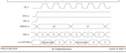
Here is the timing of the RAM configured as a single port. Since we have separate data input port (data\_a) and data output port (q\_a), it is important to understand what data you read back (old or new) from a given address during a write cycle.
