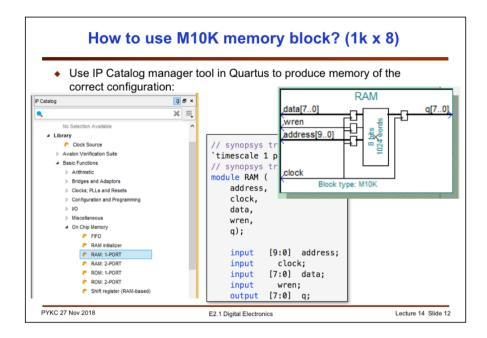
Here is an example of using the MegaWizard manager tool in Quartus. We are producing a 1-port RAM with  $1024 \times 8$ , all signals are clocked. The generator produces a sample header file (a template) which defines the interface signal to the generated block. Remember you must tick the Verilog HDL radio button.
