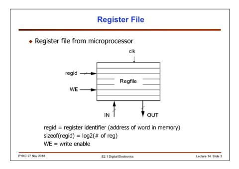
The simplest form of storage is a register file. All microprocessors have register files, which are known as "registers" in the architectural context.
