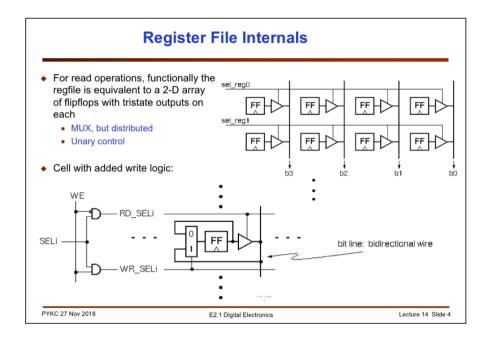
The circuit of a register file is simple – it consists of arrays of D-FFs, which can be disable (and output becomes high impedance). The register select signals sel\_reg0, sel\_reg1 etc. enable the correct register to put the data on the data line (called bit line here). The read/write control signal WE is used to determine if you are reading or writing to the register.
