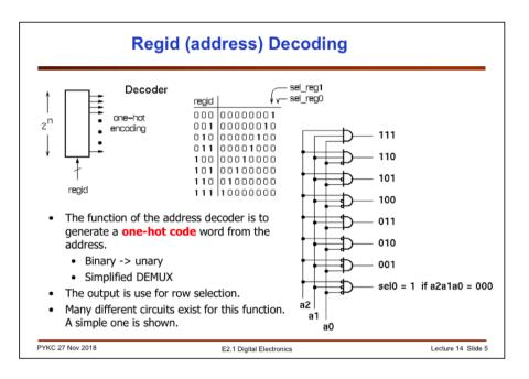
The register identification (regid) determines which register you are trying to access. This is achieved through a standard decoder, which generate a one-hot code word to select the appropriate register to access.
