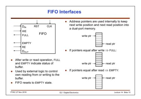
Here is a generic block diagram of a FIFO with its typical interface signals. FIFO is a form of queue. Internally there typically two counters, one keeping track of the read address (or read pointer) and another counter keeping track of the write address (write pointer). There needs to be status signals such as FULL, which is asserted if the FIFO is completely filled and writing any more words to it will destroy stored data, or EMPTY, which signifies that there are no data left to read.
