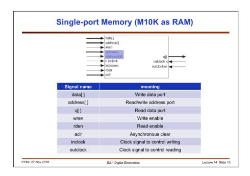
Here is a generated single-port memory with ALL possible signals included. The meaning of all the signals are self explanatory.
