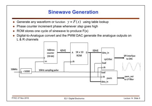
In the experiment, you have already implemented a sine wave generator using the ROM to store one cycle of a sine wave. The counter is used to advance the phase of the sine wave, which is specified as the address X of the ROM. The content of the ROM, y= F(x) is the content of the ROM and is the generated wave form. Instead of storing a sine wave, you can easily store any other signal (such as a voice or music segment).
