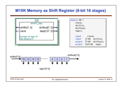
You can also configure the M9K memory block as a shift register. Here is an 8-bit 16 stage SR. In addition, it provides "tap" outputs for every stage, i.e.  $16 \times 8 = 128$  output signals. This is very useful to implement FIR filter or perform time domain convolution.
