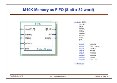
FIFO can be generated using the IP Catalog manager tool. Here is an example of a 32 word x 8 bit FIFO.
